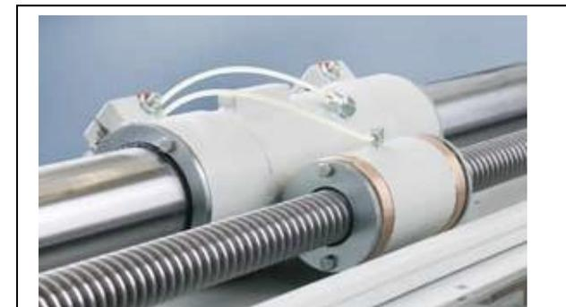
High-precision transport spindle with solid circular guide
